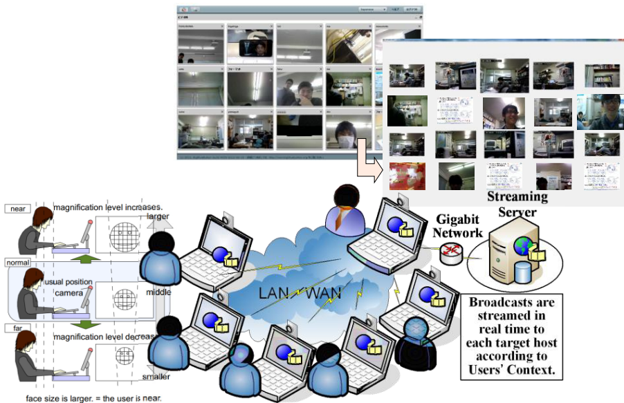
Fig. 2. Overview of GUIs for viewing student screens as thumbnails on the teacher’s computer; student screens are zoomed dynamically based on their attitude
