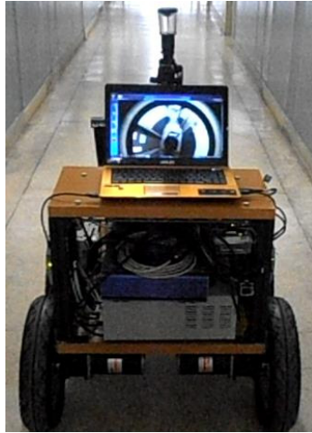
Fig. 1. An omnidirectional camera mounted on a mobile robot
