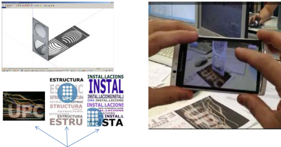
Fig. 1. AR at the UPC University. A 3D model visualized through a mobile device screen thanks to the camera detection of a regular shape or code.
