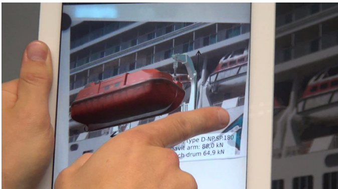
Fig. 2. AR application for the retrofitting of rescue boats and davits
