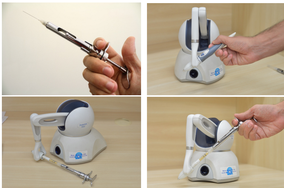
Fig. 2. Adaptation of the haptic device replacing the pen with the Carpule syringe
