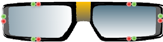
Fig. 2. Second prototype version of smart glasses having 6 green LEDs and 6 red LEDs positioned on the frames
