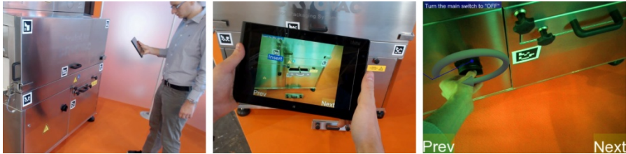
Fig. 5. Maintenance of the machine. The user frames the machine with the tablet (left) and looks at the instruction by means of the tablet (center and right).
