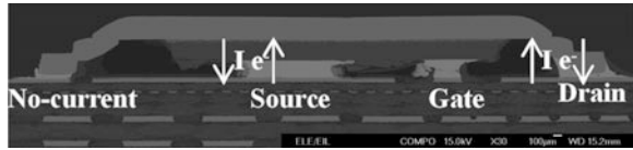
Fig. 8.25 SEM micrograph of the structure of the component used in the electromigration study
