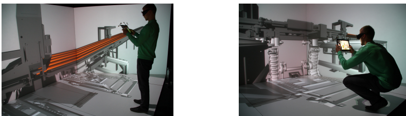
Fig. 3. A user with a tracked mobile device stands inside a virtual industrial line, which is also visible on the mobile device. The user interacts with additional AR content only accessible on the touch device. In this scenario the head of the subject, as well as the mobile device are tracked.
