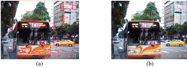
Fig. 3. Example of bus route number localization. (a) The labeled result via connected component labeling. (b) The localization result via rule-based identification method.
