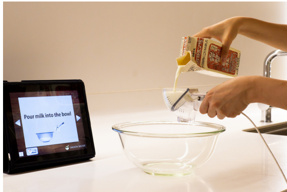
Fig. 6. Our previous work developed a utensil called “smoon,” which is a measuring spoon that automatically adjusts its capacity according to recipe data
