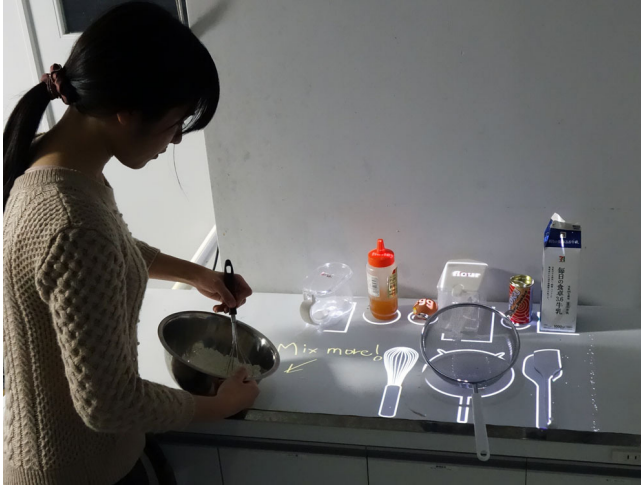
Fig. 1. An operation scene from the Shadow Cooking system. Cooking instructions are directly projected onto the kitchen counter and cooking objects. The instructions move forward according to the user's progress.
