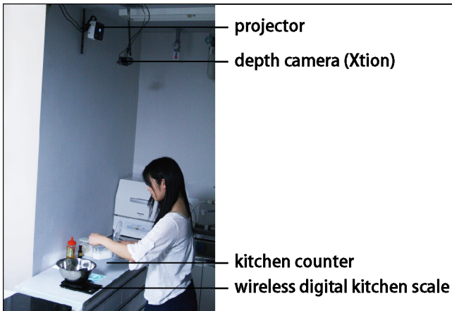
Fig. 2. Configuration of the system. The wireless digital kitchen scale tracks the quantity of an ingredient that the user has poured into the scale.
