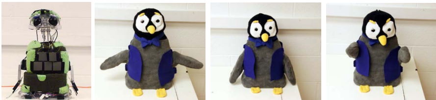
Fig. 1. Internal view of Philos and three emotional statuses (positive, neutral, and negative) represented by the eyebrow angles and hand gestures
