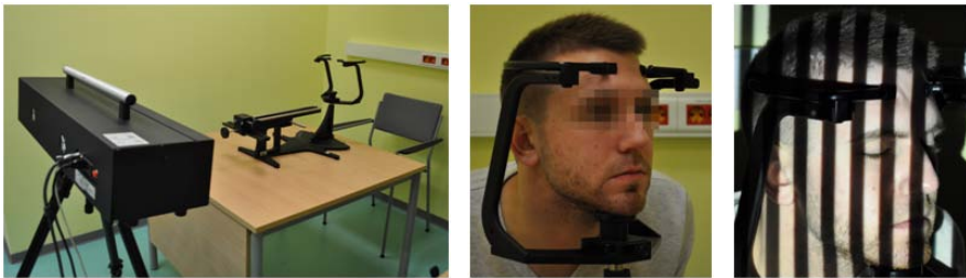
Fig. 1. Left: 3D structural light scanner. Middle: face setting with positioner. Right: scanning using the measurement stripes
