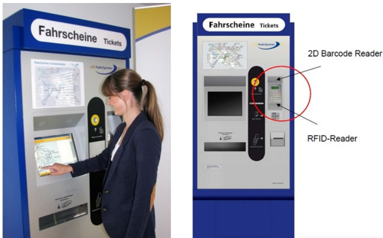
Fig. 6. Picture of a user with the TVM and diagram showing the 2D barcode reader location
