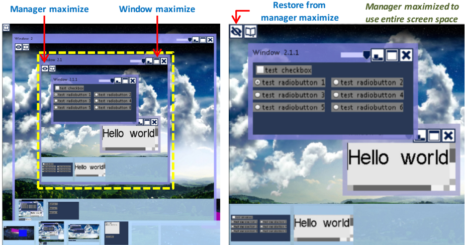
Fig. 4. Dual maximization operation applying on window managers (eye icon) and on managed windows (standard icon)
