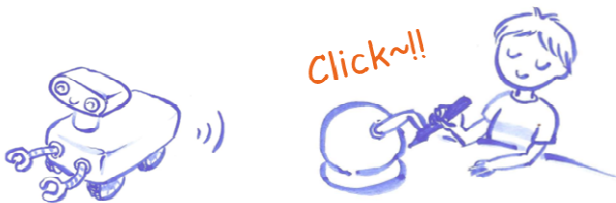
Fig. 1. The conceptual illustration of our telepresence robot with haptic visualization for individuals with visual impairments (VI) in exploring a remote environment
