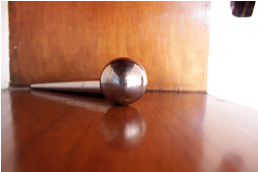
Fig. 13 Head of the femur prosthesis coated with AuNP
