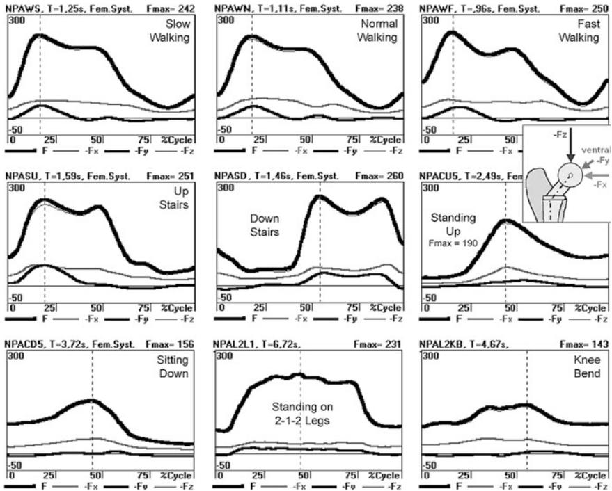
**Fig. 3** Contact force  $F$  of typical patient NPA during nine activities. Contact force  $F$  and its components  $-F_x$ ;  $-F_y$ ;  $-F_z$ ;  $F$  and  $-F_z$  are nearly identical. The scale range is  $-50-300$  % BW
