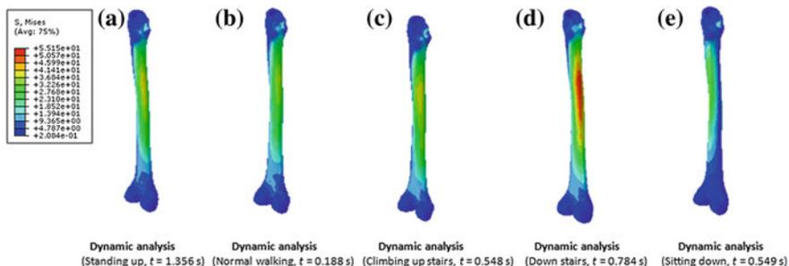
**Fig. 10** von Mises stress distribution on the bone under dynamic loading from five activities: **a** Standing up (time = 1.356 s), **b** Normal walking (time = 0.188 s), **c** Climbing up stairs (time = 0.548 s), **d** Down stairs (time = 0.784 s) and **e** Sitting down (time = 1.549 s)
