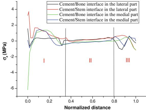
**Fig. 13** Variation of the normal stress according to  $y$ -direction ( $\sigma_y$ ) along the cement/bone and cement/stem interfaces in the different sides (lateral and medial) of the cement mantle for the static and dynamic analysis (down stairs, time = 0.784 s) *I* Proximal part, *II* Median part and *III* Distal part
