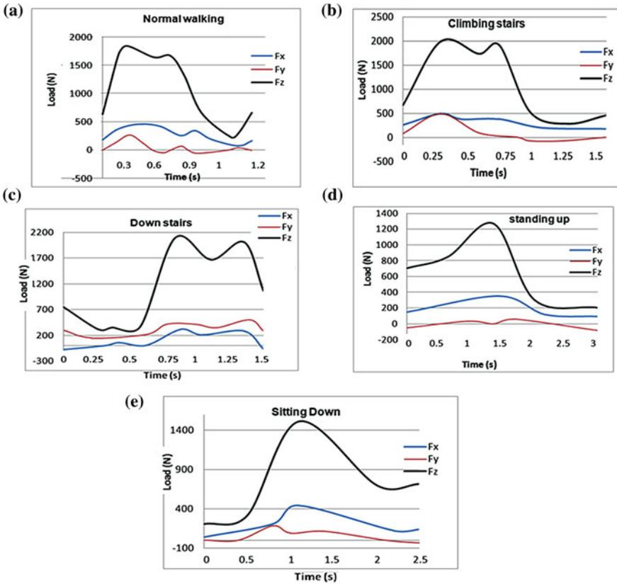
**Fig. 4** The variation of forces applied on the prosthesis during five activities (**a** walking, **b** climbing up stairs, **c** down stairs, **d** standing up and **e** sitting down) for BW = 70 kg
