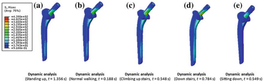
**Fig. 8** von Mises stress distribution on the implant under dynamic loading from five activities: **a** *Standing up* (time = 1.356 s), **b** *Normal walking* (time = 0.188 s), **c** *Climbing up stairs* (time = 0.548 s), **c** *Down stairs* (time = 0.784 s) and **d** *Sitting down* (time = 1.549 s)
