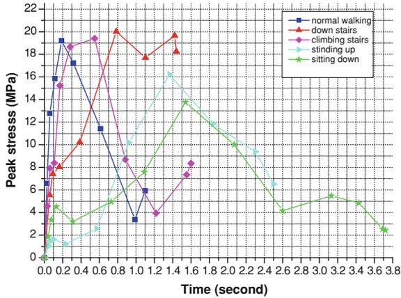
**Fig. 7** Maximum von Mises stress in the cement mantle during five activities: *Standing up* (time = 1.356 s), *Normal walking* (time = 0.188 s), *Climbing up stairs* (time = 0.548 s), *Down stairs* (time = 0.784 s) and *Sitting down* (time = 1.549 s)
