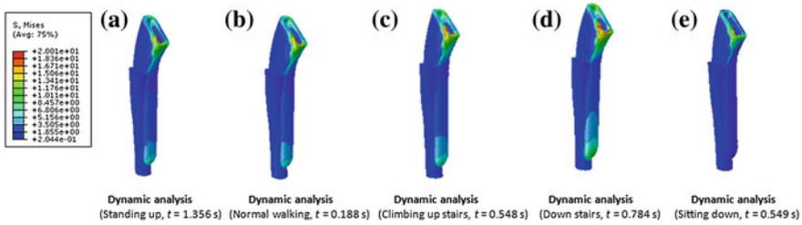
**Fig. 6** von Mises stress distribution on the cement under dynamic loading from five activities: **a** Standing up (time = 1.356 s), **b** Normal walking (time = 0.188 s), **c** Climbing up stairs (time = 0.548 s), **d** Down stairs (time = 0.784 s) and **e** Sitting down (time = 1.549 s)
