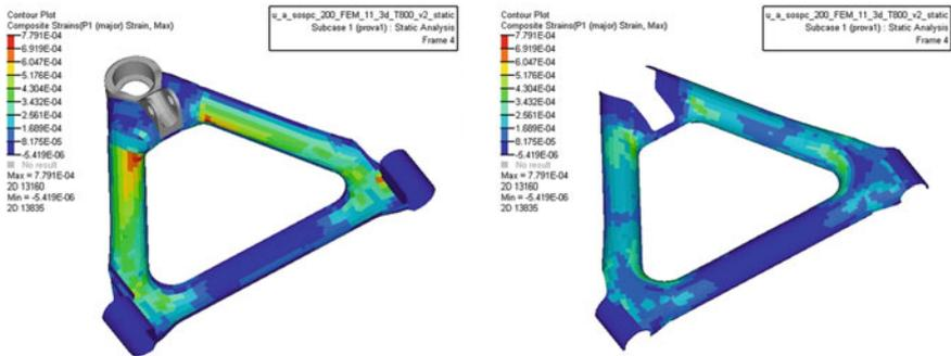
Fig. 10 Static strain of the upper wishbone arm (*upper and lower shell*)
