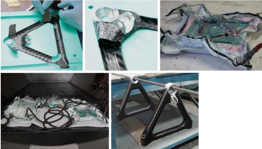
**Fig. 11** Production sequence of upper wishbone
