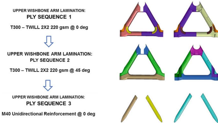
Fig. 6 Lamination sequence for the upper wishbone
