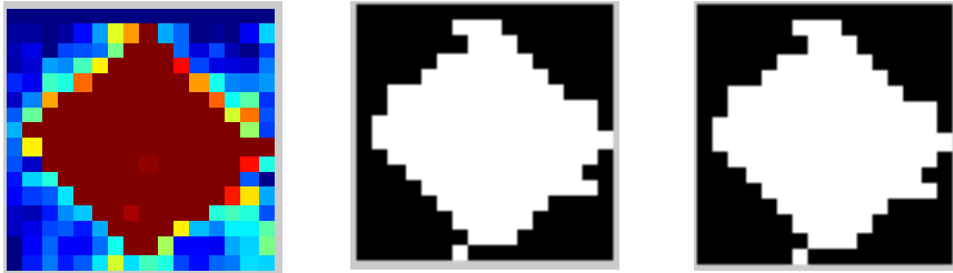
Fig. 3. (a) 8 bit tactile image of square object; (b) Tactile image after convolution and thresholding ; (c) Final image after morphological operations
