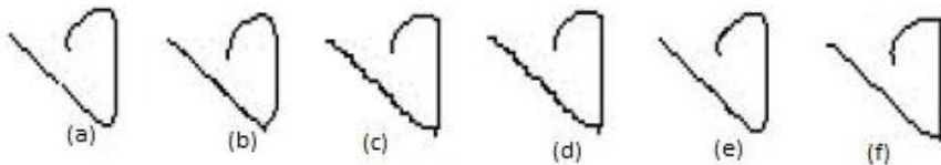
Fig. 3. Skeleton of e (ଏ) by algorithms (a) CCS (b) CWSI (c) KGK (d) ZS (e) ZW and (f) proposed algorithm
