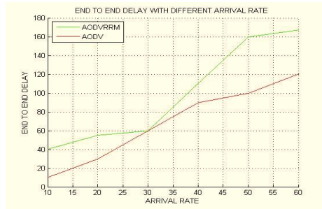
Fig. 4. End-to-End delay vs arrival rates
