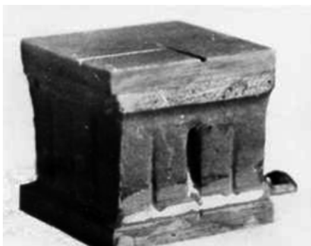
Fig. 13.1 The thermoelectric battery for RTG “Life.” Temperature gradient 320–850 K, efficiency 10 %
