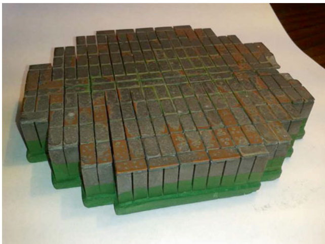
Fig. 13.1 The thermoelectric battery for RTG “Life.” Temperature gradient 320–850 K, efficiency 10 %
