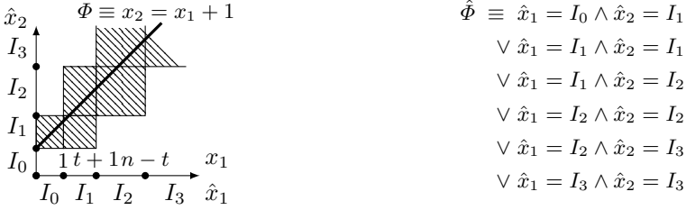
Fig. 7. The shaded area approximates the line x_2 = x_1 + 1 along the boundaries of our parametric intervals. Each shaded rectangle corresponds to one conjunctive clause in the formula to the right. Thus, given \Phi \equiv x_2 = x_1 + 1 , the shaded rectangles correspond to \|\Phi\|_{\exists} , from which we immediately construct the existential abstraction \hat{\Phi} .
