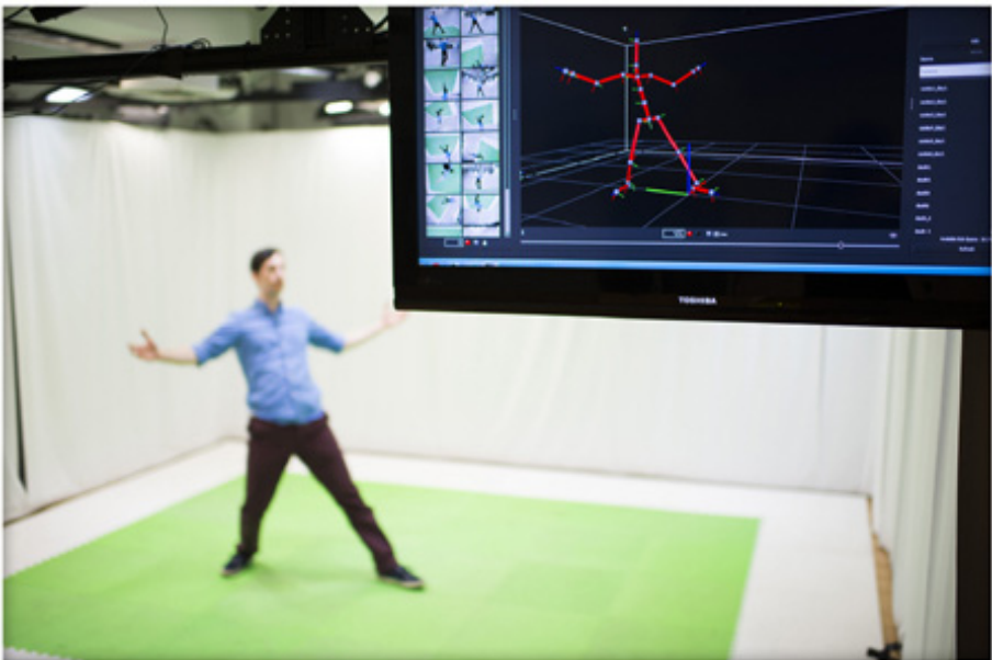
Fig. 2. OpenStage® V2.0 Markerless Motion Capture System ( source: Organic Motion )
