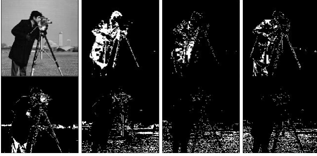
Fig. 2. The original Cameraman is illustrated in the upper Left Hand Side (LHS). Binary masks of the layers of the Cameraman are plotted in increasing intensity from left to right (e.g., \{(row, column)\} = \{(1, 2), (1, 3), (1, 4), (2, 1), (2, 2), (2, 3), (2, 4)\} ). 7 of 16 layers are illustrated. White denotes a pixel is present in that mask; black denotes it is not present. The lower pixel intensity values form the cameraman; cameraman parts are low frequency –the pixels are regionally activated in plot (1, 2) & (1, 3). The cameraman outline is captured in layer (1, 4), which captures edges. Plot (2, 1) captures the cameraman’s trousers, which are a low frequency region. The remaining layers capture high frequency background.
