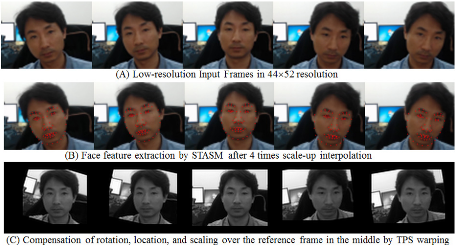
Fig. 2. TPS warping process. The middle column is a reference frame and the others are data frames.
