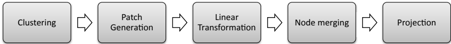
Fig. 1. The original graph is first partitioned into clusters which are then used to create overlapping patches. For each pair of overlapping patches a linear transformation is computed that brings shared nodes together. They are then merged before they are projected into screen space.
