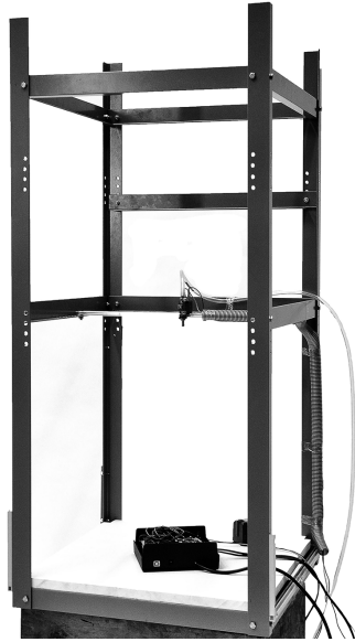
Fig. 3. The SyncBox main equipment. Devices shown on the shelf, the synchronizer box (black) and the pump (gray, partly behind framing) are normally placed aside, as a water container is placed here instead. In the middle part of the framing, the valve can be seen.
