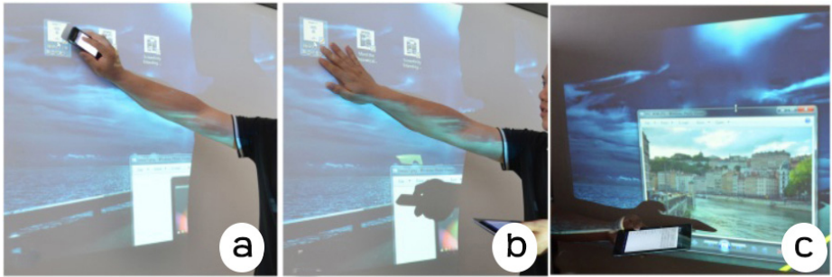
Fig. 4. Interactions in PrZ (a: user selects a file with smartphone and downloads the file, b: user selects a file by hand, and clicks on the tablet to download the file, c: upload an image from the tablet to the screen)
