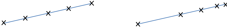
Fig. 1. TSP with uniform speed (left) and deceleration (right). All positions are sampled with the same frequency.
