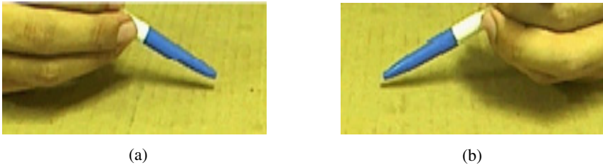
Fig. 11. Varied saturation of the produced shadow: (a) a more saturated shadow (the pen tilt angle = -63.43^\circ ); (b) a less saturated shadow (the pen tilt angle = 63.43^\circ )
