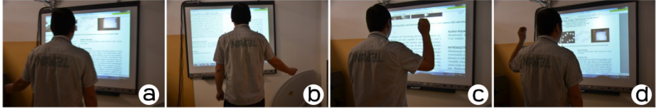
Fig. 2. Gestures Available in EZ (a: scroll up, b: scroll down, c: zoom in, d: zoom out)
