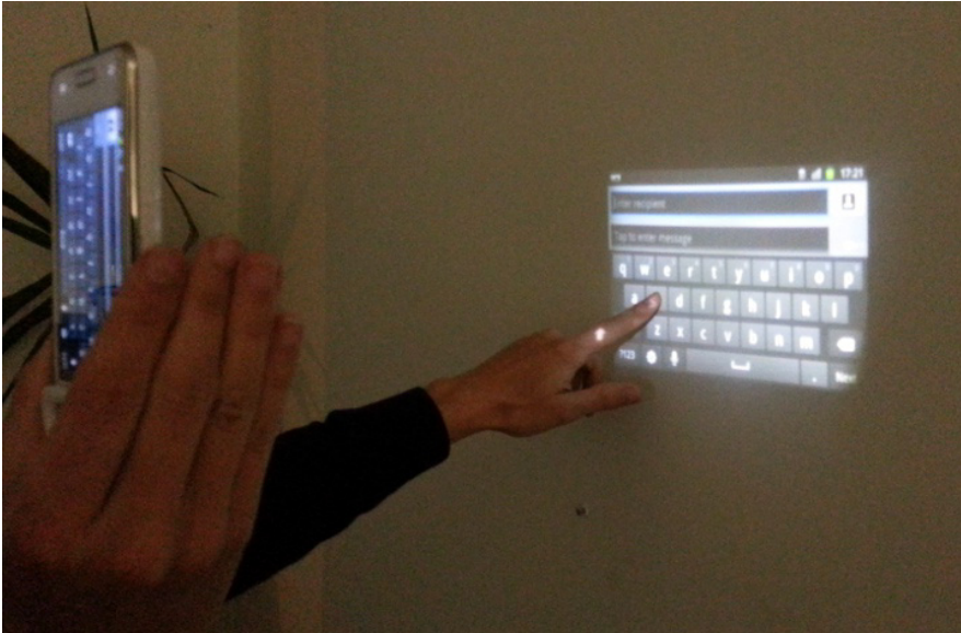
Fig. 1. In our approach, we use a smartphone with an integrated projector and a built-in RGB camera. The user holds the smartphone in one hand and projects the screen content onto a planar surface, while the camera is used to detect the projected screen and the user's interaction with it. The detected hand motion and gestures are forwarded to the smartphone's operating system as touch input events.
