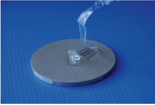
Fig. 22.3 Antibacterial-loaded, fast-resorbable, hydrogel coating (DAC ® , Novagenit ® , Mezzolombardo, Italy) spread on a sanded titanium disk. The coating, that has received the CE mark and is available for clinical use in Europe, has been proved effective to inhibit biofilm formation on different substrates in vitro and to prevent implant-related infection in a rabbit model of implant-related infection
