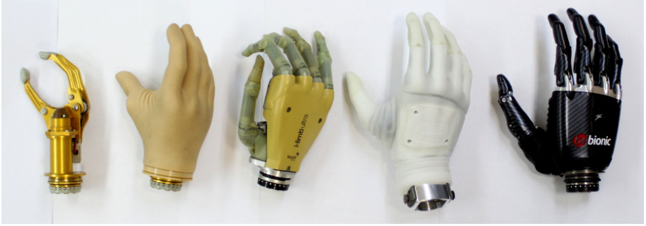
Fig. 1. Two basic hand prostheses on the left compared to more current hand prostheses like the i-limb TM ultra, Michelangelo TM and bebionic3 TM hands
