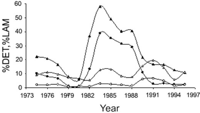
Fig. 10.30 %DET (black circles) and %LAM (black triangles) of waiting time sequences from the declustered Central Asia EQ catalogue (1975–1996) at a representative threshold of M > 2.5 . Window length is 500 days with sliding step size of 100 days. Open symbols correspond to randomized data sets showing attenuation of deterministic structures
