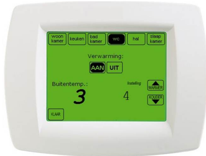
Fig. 3. The simulated programmable heating system interface
