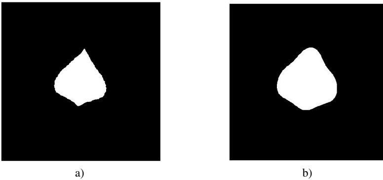
Fig. 3. a) Original image, b) Reconstructed image from Zernike Moments
