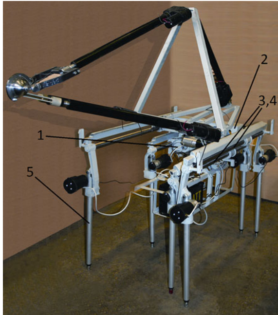
Fig. 1 Walking mobile robot with manipulator-tripod: 1 bottom body; 2 top body; 3, 4 guide blocks; 5 vertical adaptation drives
