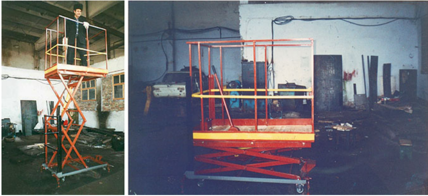
Fig. 2 Experimental specimen PMD-2.2. In raised and transport positions
