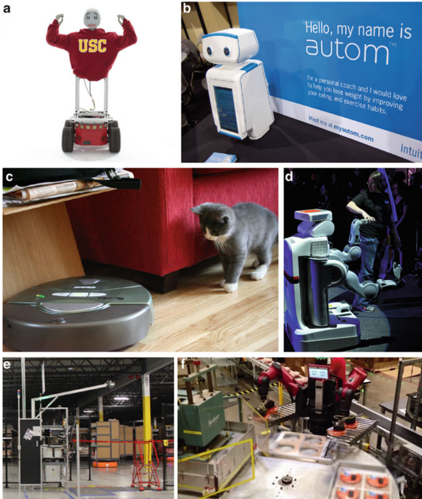
Fig. 1 Examples of co-robots from the domains of socially assistive robotics ( top ), domestic service ( middle ), and cooperative manufacturing ( bottom ); not shown to scale. (a) USC's Bandit provides several types of hands-off guidance, including physical exercise activities for seniors and stroke patients. (b) Intuitive Automata's Autom is a personal weight loss coach. (c) iRobot's Roomba is a commercially available robot vacuum; appliance robots designed solely for floor cleaning are the most successfully adopted home-use robot. (d) Willow Garage's PR2 is capable of various household chores, including folding laundry. (e) KIVA Systems' orange drive robots transport warehouse merchandise to inventory station, where human workers "pick" items for order fulfillment. (f) Rethink Robotics' Baxter unloads newly vacuum sealed packages from its station at a rotary table while adjacent human workers reload the molds
