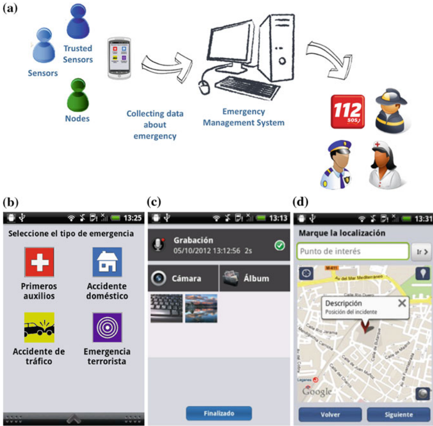
Fig. 2 Collecting data from human sensors a System architecture b Crisis selector c Multimedia manager d Map position
