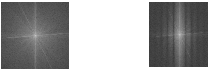
Fig. 1. Vizualization of discrete FT results before and after artificial distortion by horizontal blurring center
