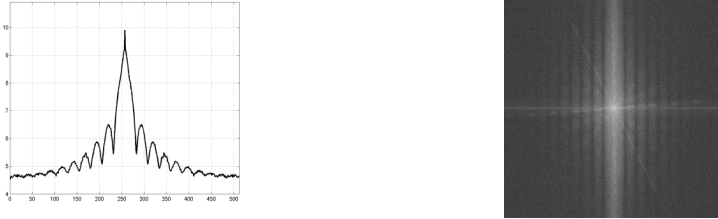
Fig. 4. Visualization of discrete FT results for the image with artificial horizontal blur of 20 pixels
