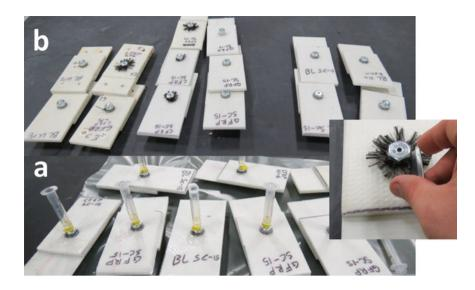
The adherend/plates were joined using ordinary grade 8 nominal 1/2 in. bolts and matching flat washers. Conventional bolted joints had no insert, and the bolts were not drilled. Bolts with drilled 2 mm diameter passageways for resin injection were used for the remaining specimens. All the bolts were torqued to 35 N m.
