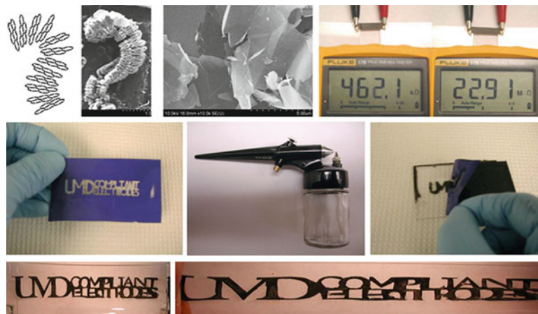
Fig. 8.1 (Top) Schematic illustration of separation of the layers in graphite by exfoliation, SEM images of exfoliated graphite (EG) showing mixtures of sheets of graphene and multi-layer graphite, and latex strain sensors. (Center) Deposition and patterning by spray coating through a stencil. (Bottom) Compliant electrode/sensor material on a compliant substrate
