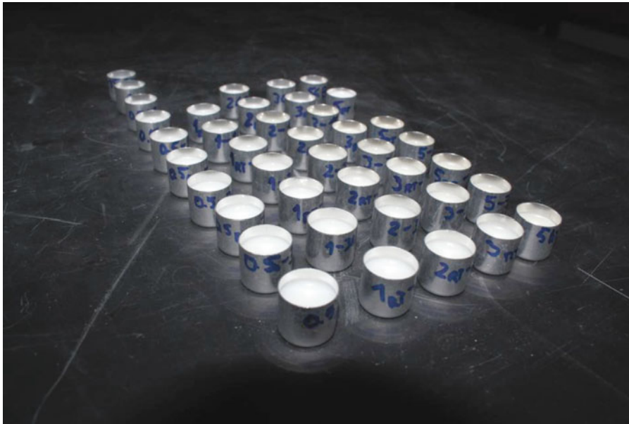
Fig. 20.1 Micro- and nano-modified epoxy resin samples prepared for volumetric measurements
