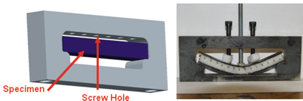
Fig. 13.1 The fixture to shape the sandwich composite through heat treatment to fabricate sandwich composite with constant curvature
