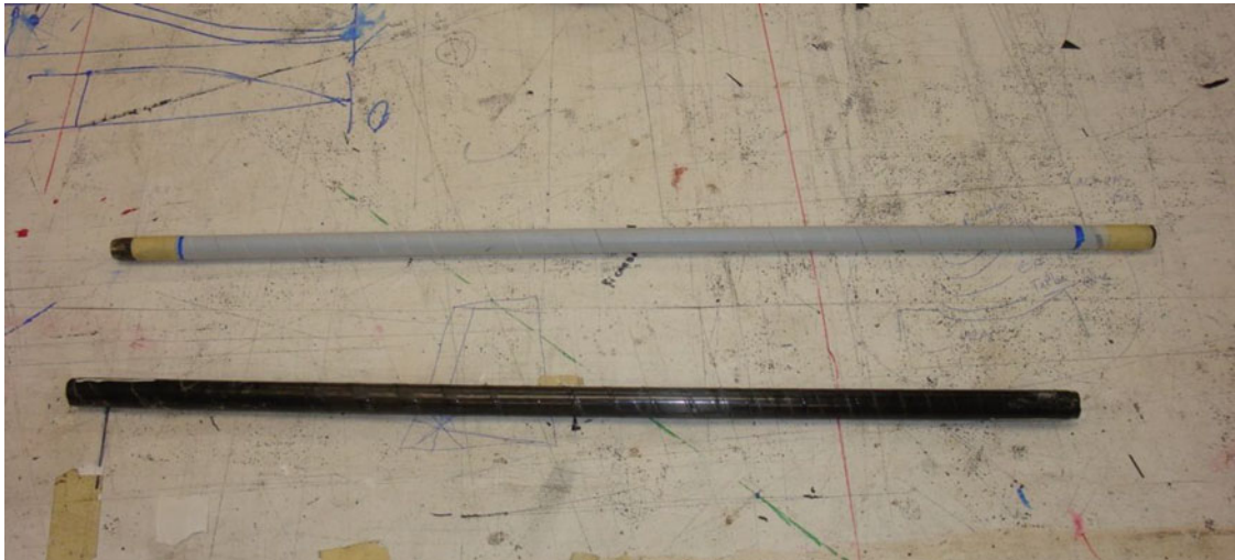
Fig. 15.4 The steel mandrel wrapped in non-stick Teflon. Beneath that is a completed carbon fiber shaft 18 \frac{1}{2} " in length
