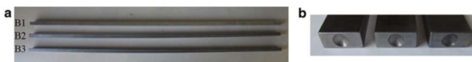
Fig. 8.1 (a) Specimens with different initial curvatures and (b) detail of end cross-sections with spherical cavities
