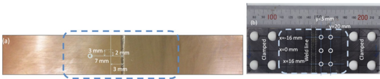
Fig. 15.1 Butt-welded specimen 1 (a) and specimen 2 (b). The box with dashed lines indicates approximate area of view. For specimen 2 strain was measured with strain gauges at 12 points; 5 mm and 20 mm away from the weld line along the tensile axis, 16 mm above/below the central line parallel to the tensile axis. Circles indicate these locations for the right side of the weld line only. Strain gauge measurements were made on the left side of the weld line at the locations symmetric to these six points. The circle and distances inserted in (a) indicate the locations where acoustic velocity is previously measured in a welded specimen similar to this study
