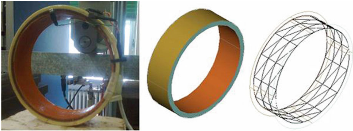
Fig. 29.1 Dedicated loop antenna ( left ) with its CAD representation ( right )
