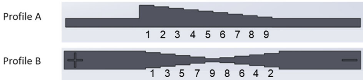
Fig. 9.2 Numbered profile steps by cross-sectional area thickness (1 represents the thickest while 9 represents the thinnest cross-sectional area)
