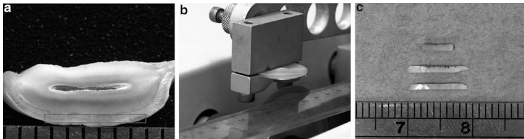
Fig. 5.2 (a) Slice of cervine enamel was cut by (b) low speed saw to make (c) enamel specimens for bending tests
