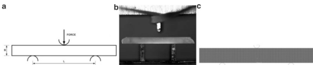
Fig. 5.3 (a) Schematic and (b) experimental setup of three points bending ramp-hold test and (c) corresponding FEA model
