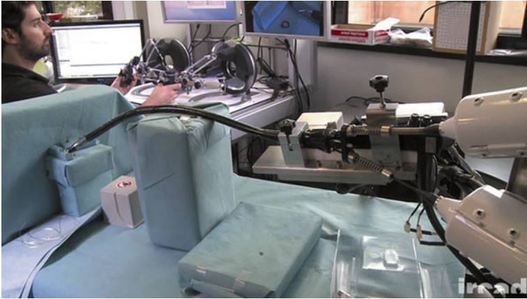
Fig. 1.2 The robotic version of the ISSSCOPE® (Courtesy of Karl Storz, Tuttlingen, Germany) is telemanipulated through an intuitive haptic interface that allows for very smooth and controlled micromovements
