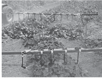
Fig. 1 Directed spray application of mycoinsecticide using conventional spray equipment that directs most of the spray into the cucurbit canopy. ( Top ) Spray designed to treat two rows of cucurbits. ( Bottom ) Close-up of drop tube and nozzle arrangement. Note height of nozzles in relation to plant canopy and rearward direction of spray. (Reprint from Fig. 1 in Jaronski (2010).)
