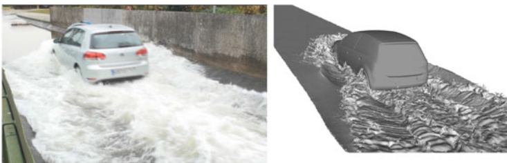
Fig. 3 Experiment ( left ) and simulation ( right ): Rear view of the vehicle at 4 s
