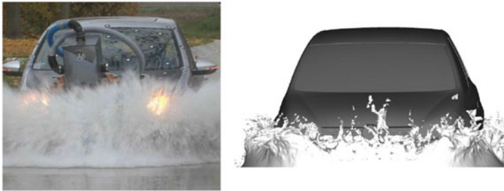
Fig. 2 Experiment ( left ) and simulation ( right ): Front view of the vehicle at 4 s
