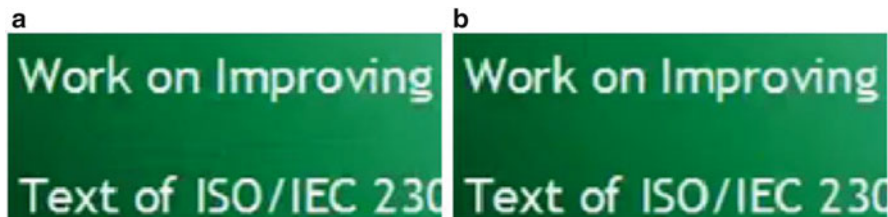
Fig. 7.24 Example of test sequence SliceEditing in LP condition, POC = 100, QP = 32: (a) SAO is disabled, (b) SAO is enabled
