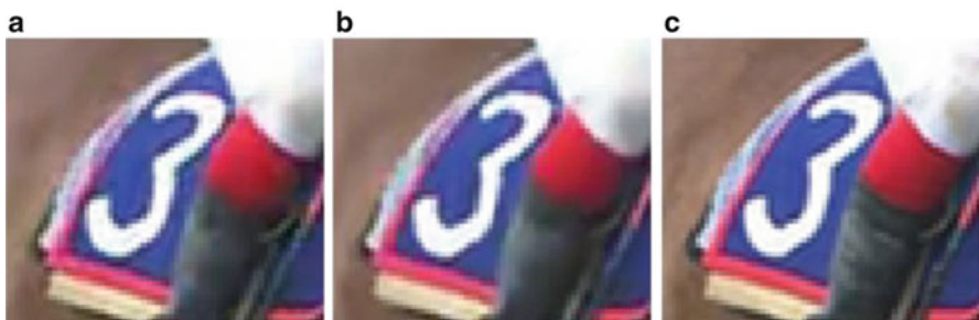
Fig. 7.25 Subjective quality comparison of RaceHorses test sequence, POC = 20, QP = 32, LP condition: (a) SAO is disabled, (b) SAO is enabled, (c) original (uncoded) sequence
