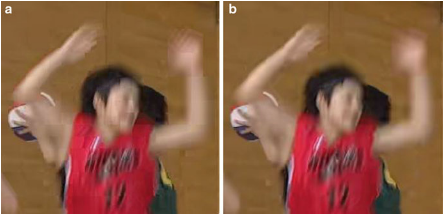
Fig. 7.22 Sequence BasketballDrive , Random Access, QP32: (a) deblocking turned off, (b) deblocking turned on
