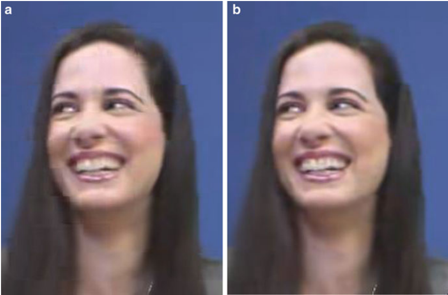
Fig. 7.23 Sequence KristenAndSara , Low Delay, QP37: (a) deblocking turned off, (b) deblocking turned on
