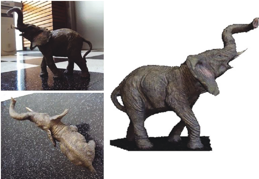
Fig. 6 Two out of 21 input images of the elephant model data set ( left ) and the resulting 3D reconstruction ( right )
