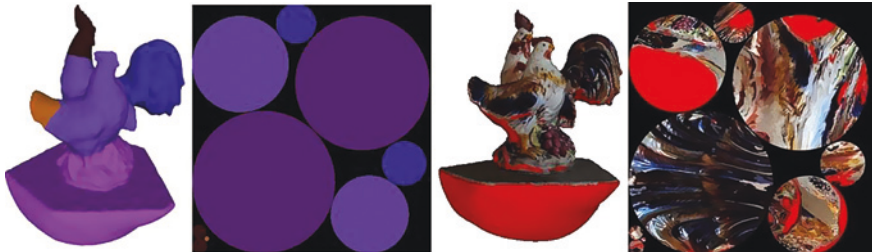
Fig. 2 The Rooster model: the segmented 3D model and the corresponding texture atlas ( left ) and the reconstructed texture obtained by projecting and fusing input photographs ( right )
