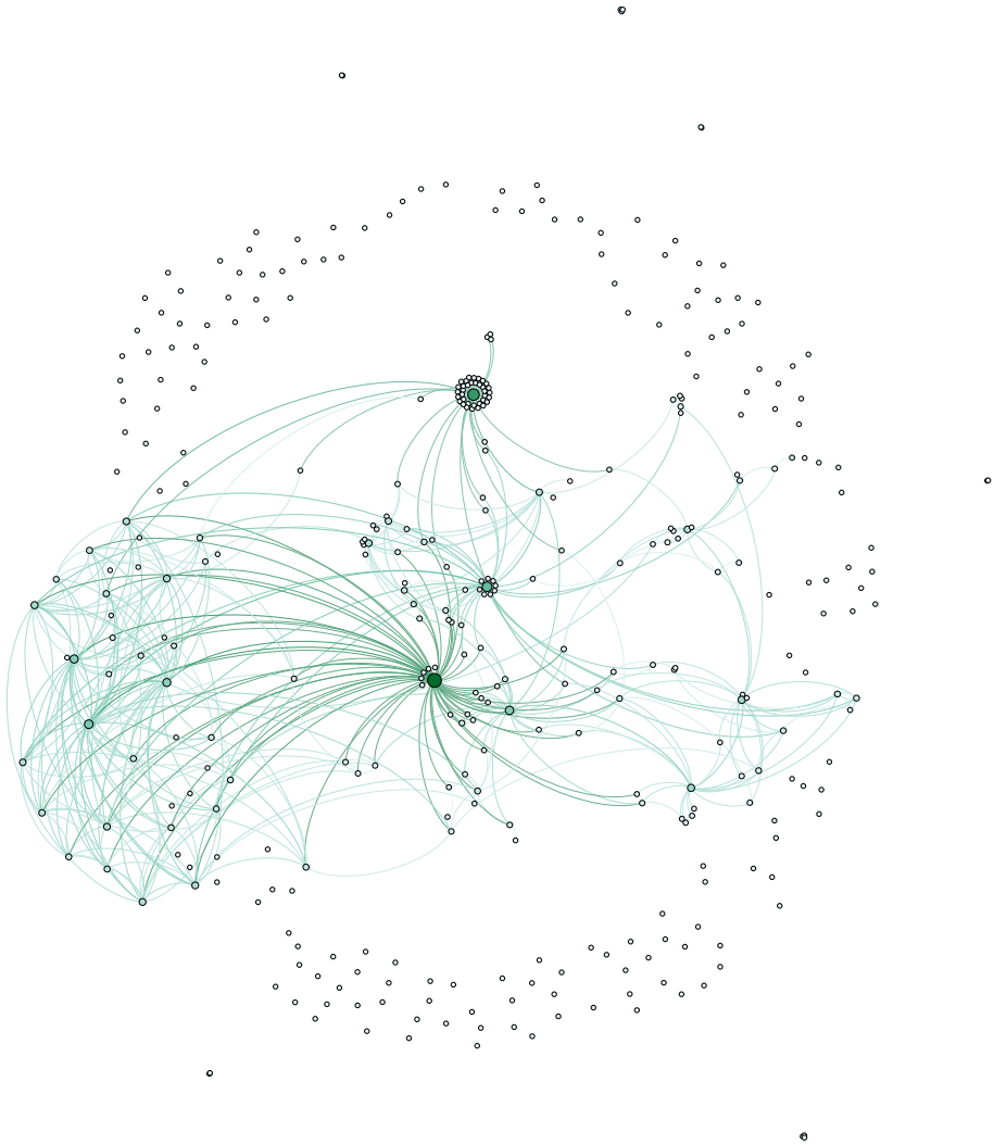
Fig. 3. Dependency network for Eclipse Kepler. The size and shade of nodes are proportional to their degree.
