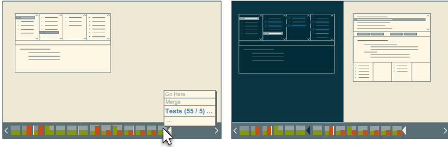
Fig. 5 The items in the version bar are now a visualization of the results of the tests that have been run in the background ( left ). A second inner environment allows the user to explore a previous version next to the current one ( right )
