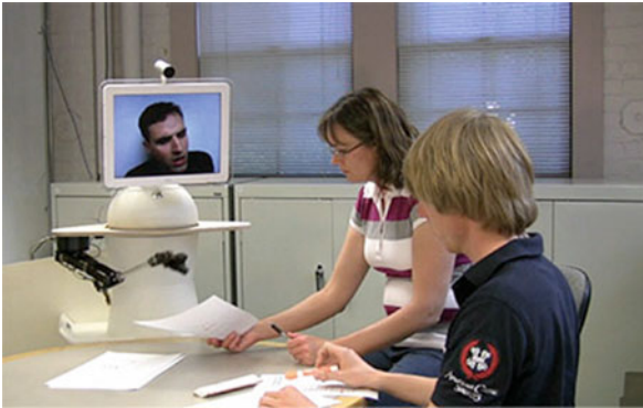
Fig. 2 Video prototype of the crowdsourced robotic telepresence study. An initial study found that perceptions improved when the remote person's onscreen actions and the robotic platform's in-space movements were consistent. The study used Wizard of Oz to actuate the robot: initially using manual levers, and later using remote teleoperation
