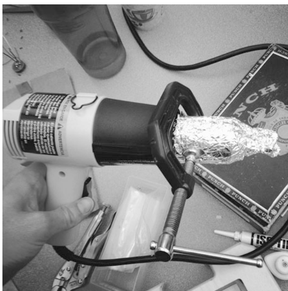
Fig. 2 Low fidelity prototype of an improved heat gun design
