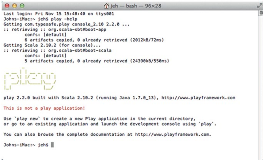
Fig. 38.4 Testing the Play Framework installation
