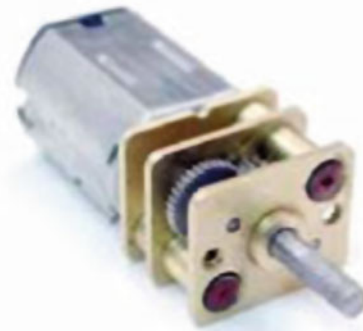
Fig. 8 Solarbotics motor and gearbox assembly used in MiLyBot [52] (copyright @ 2008 Luis Vegas et al.)
