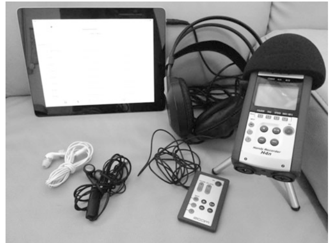
Fig. 2 The hardware used for the experiment and survey. (1) Apple iPad used to play back the signals, (2) AKG K99, Zoom H4n with remote, consumer headphones (Samsung and HTC)
