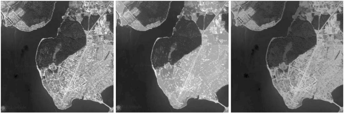
Fig. 2 Illustration of the effect of an area closing and area opening to satellite images. Images from left to right : original image, result of area closing, result of area opening
