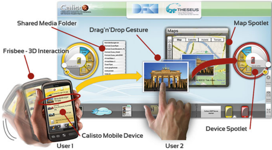
Fig. 4 Types of touch interaction in the CALISTO system. The user can use touch gestures to interact with spotlets. Data can be “thrown” (transferred) with the “frisbee gesture” from a mobile device to the stationary display
