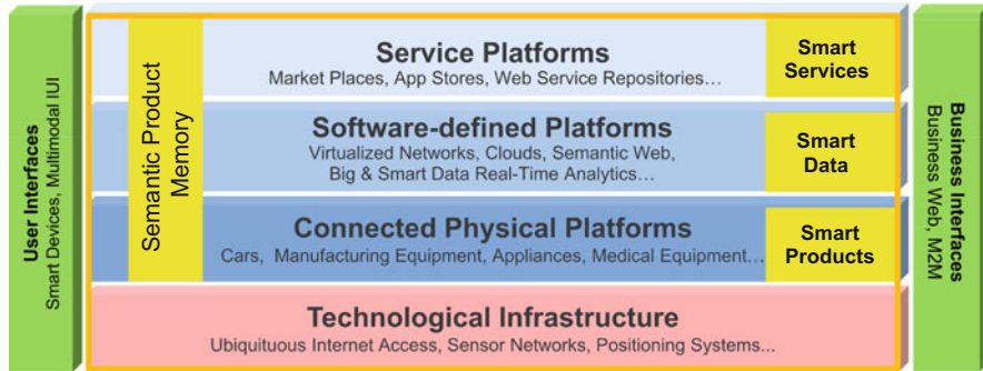
Fig. 5 Platform stack for customized smart products, data and services
