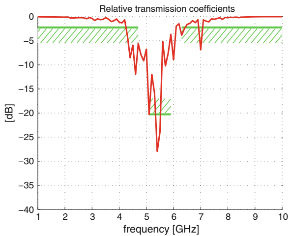
Fig. 4 Transmission coefficients of the optimized FSS Wi-Fi filter where \theta = 15^\circ (angle of incidence)
